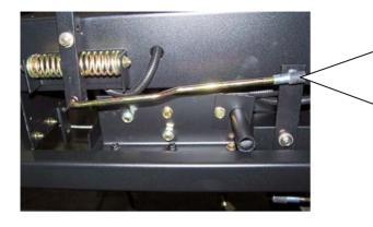
Once both hydro units are pulling equally, make your final control handle adjustment with this ball linkage. Whichever handle is going the farther forward, lengthen the linkage on that side until the handles are straight across when mower is traveling in a straight line. If a lot of adjustment is needed, shorten the linkage on the opposite side for half of the adjusting.
